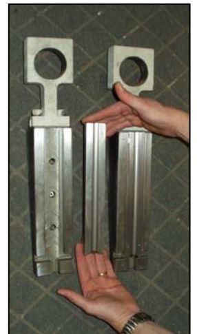
Fig 2. Anti-rotational device fitted to the test platform to prevent the piston from spinning as the cable unwinds.
