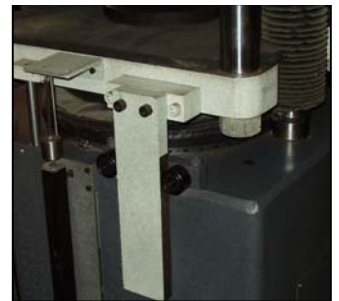
Fig 2. Anti-rotational device fitted to the test platform to prevent the piston from spinning as the cable unwinds.
