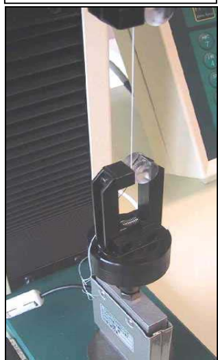
Elastomer Fibre tests using pneumatic grips
