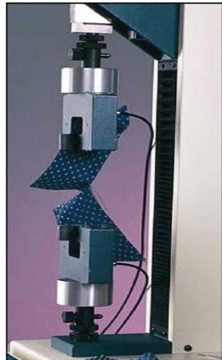
Tear Tests using Pneumatic grips
