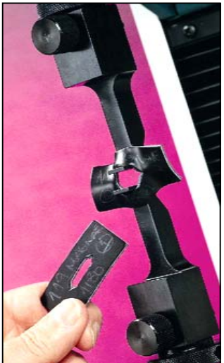
Leather Tests (tear)
