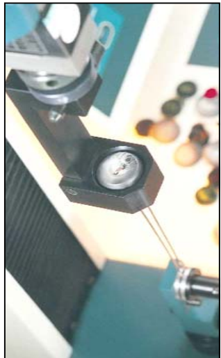
Button Break tests
